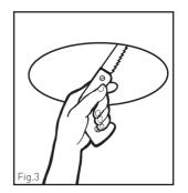
3. Use an electric jig saw or small hand saw to cut out around this line. Several holes drilled at a point inside the circle provides a convenient starting point for cutting the panel out.
