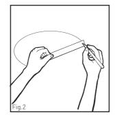
2. Use the template provided to draw a circle 300mm in diameter. To do this insert a thumb tack in hole at one end and insert a pencil in the other hole and scribe a circle.
