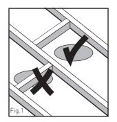
1. Determine the position in ceiling where fanlight is required to be installed. (Do not install within 120cm of stove or inside a shower recess). Be certain that the installation area is not restricted by roof beams above a ceiling refer table for clearance required
