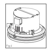
4. Remove the terminal cover and wire according to the diagrams in section 2.
