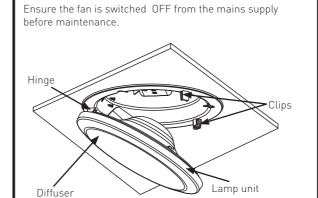
■ Hold on to the "Lamp Unit" on opposite side of Hinge as shown and pull down firmly to release the Lamp Unit for cleaning. After cleaning assemble the Reflector unit by locating the 2 x Latches in the clips and push up gently until you hear a "Click".
